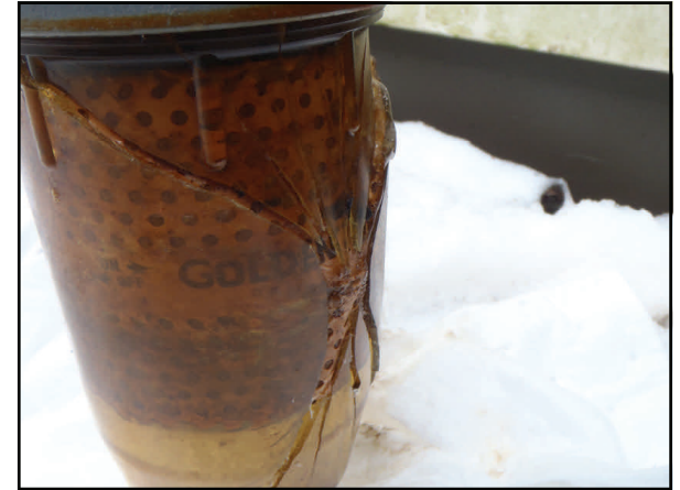
Check your tank for water! Water can corrode a tank from the inside out or cause the fuel filter to crack during cold weather. (Photo)
